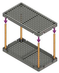
Slide the **axles** (dowels attached to wheels) through the frame, two holes from the bottom.
