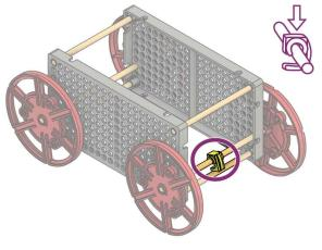
8 Insert a 13 cm (5 in) dowel through the frame and a rubber band, as shown.
