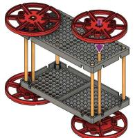
) Tap or push another hole plate onto the dowels to finish your frame.
