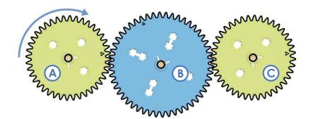
A gear inserted between two or more gears is known as the **idler-wheel**. It works to keep the direction of rotation of the input and output gears the same, without affecting **gear ratio**.
