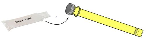
A small amount of silicone grease will lubricate many plungers (a 1cc packet can lubricate over 30 pistons). Save the extra lubricant to use later.
