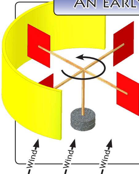
The Persian windmill was used around 1000 b.c. to turn a grindstone. It is the oldest known windmill design. The machine works by blocking the wind blowing on  $\frac{1}{2}$  of its sails. The sails exposed to the wind are pushed downwind due to drag, causing the windmill to rotate.
