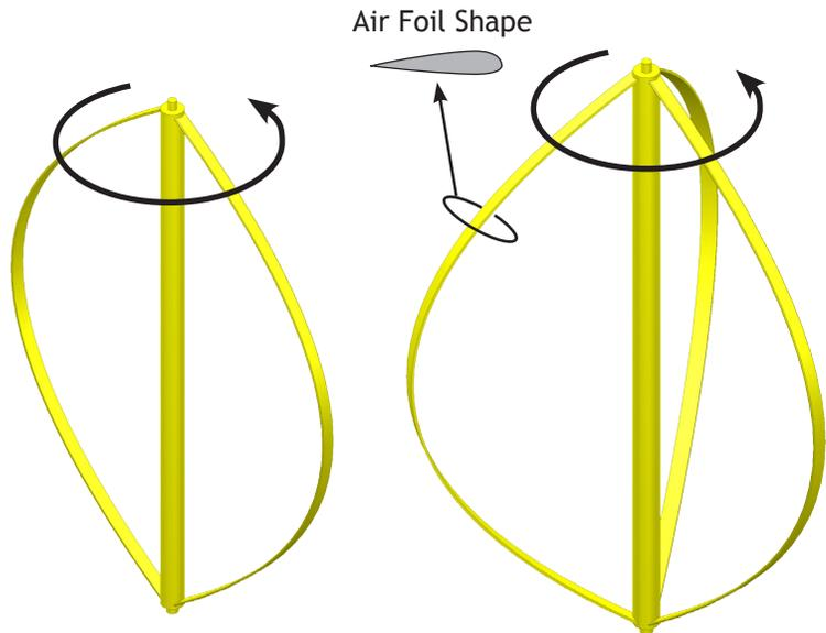
The Darrieus turbine is not self starting. It needs to start turning before the wind will begin rotating it.
