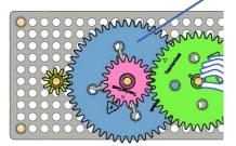
Compound gears are two gears on the same axle.
