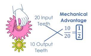
When mechanical advantage is less than 1, force goes down (and speed goes up).
