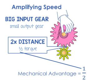
Find mechanical advantage using the gears' teeth.
