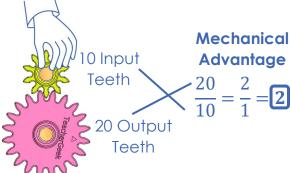
When mechanical advantage is bigger than 1, force goes up (and speed goes down).
