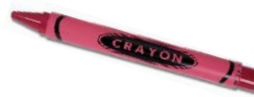
Crayon (rub on dowels to make sliding them easier into holes of components)
