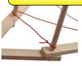
Cables can be secured to dowels at joints.
