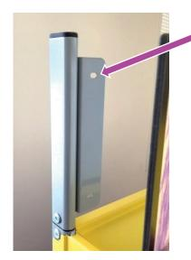
Holes for mounting the sign to the cart.
