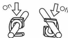
Press a **stop clip** onto a **dowel** to keep it from sliding or use it as a hook for a string / rubber band. It takes little force to get it on.
