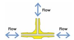
T-Connectors: allow fluid to flow between three ports (openings).
