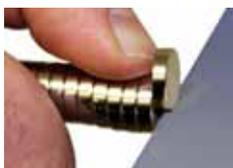
Magnets can be removed by gently pushing them up and out with a straight screwdriver.
